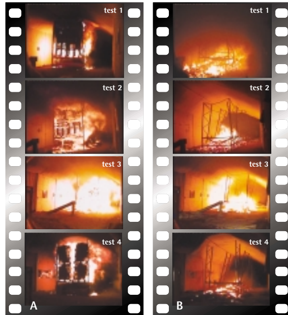
Figure 12 Overview of fire development. A After 5 minutes B After 30 minutes
