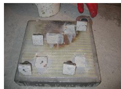
Bonding strength test after combustion test
