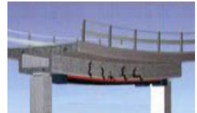
Installation of CAFT System
