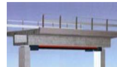
Increasing load rating after CFRP tensioning
